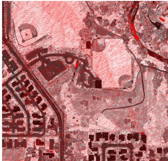
Figure 4. Image produced using LIDAR intensity data for first returns. Red pixels in the image indicate areas where there were no first returns within the pixel. LIDAR data were acquired at a density of 5.5 pulses/m 2 (0.43 m between pulses) using a pulse size of 0.33 m (average diameter at ground level). Image pixels are 0.45 by 0.45 m. Image represents an area that is 434 m wide and 411 m high.
